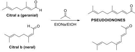
Figure 2. Synthesis of pseudoionones via aldol condensation
