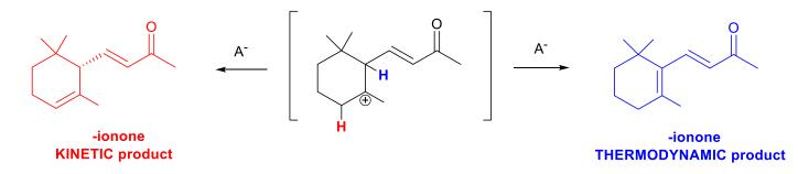
Figure 5. Formation of different alkenes in ionone isomers
