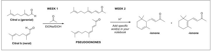
Figure 7. Reaction schemes for ionone synthesis from citrals
