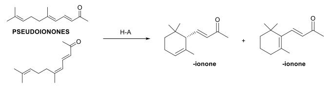
Figure 3. Acid-catalyzed cyclization of pseudoionones
